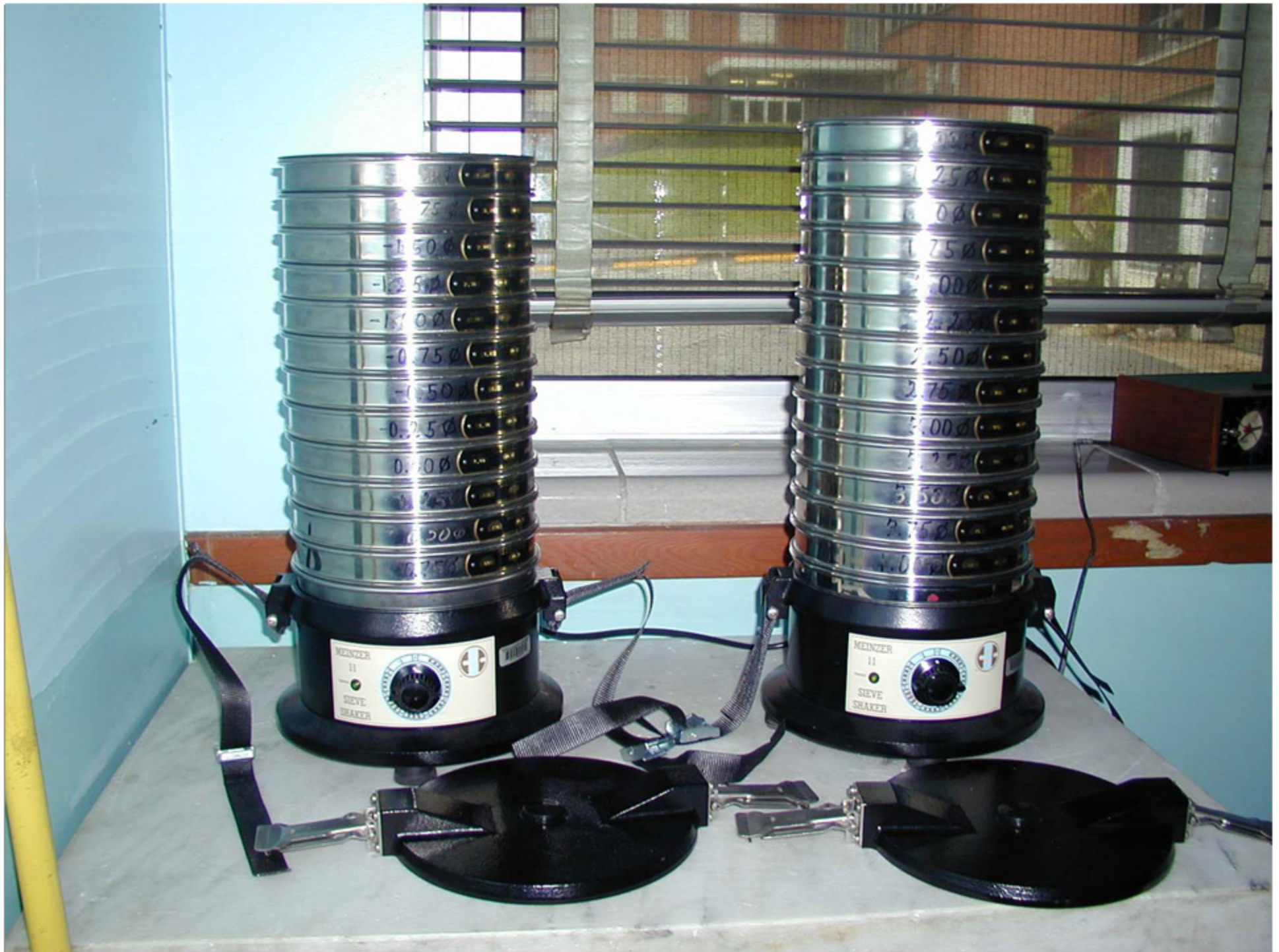
Figure 6. Sieve Nest Used in Processing Sediment Samples
