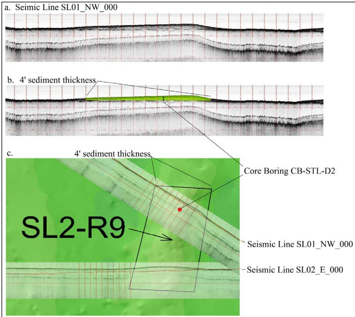
Figure 5. a. Seismic line SL01\_NW\_000 showing a surficial shoal offshore of St. Lucie County elucidating the triangular nature of the source. b. Boring CB-STL-D2 is projected on the seismic line along with the extents of the source horizontally to a 4 foot thickness. c. The planer extent of the source is outlined as identified using the seismic and bathymetric data.
