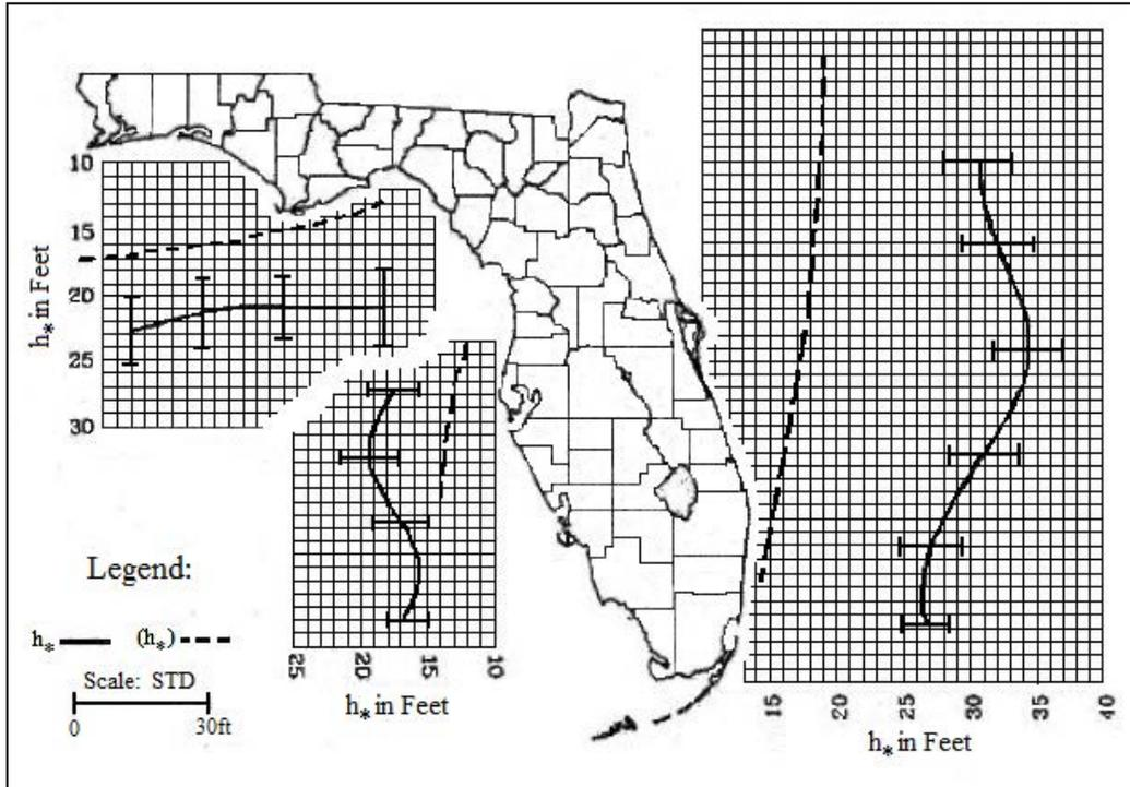
Figure 4. Depth of closure was selected for the study areas from Dean and Malakar (2002). Depth of closure calculated from Dean and Malakar (2002) are represented by  $h_*$  with a solid line compared with depth of closure determined by Dean and Grant (1989). The vertical bars represent  $\pm$  one standard deviation about the averages of the depth of closure values.
