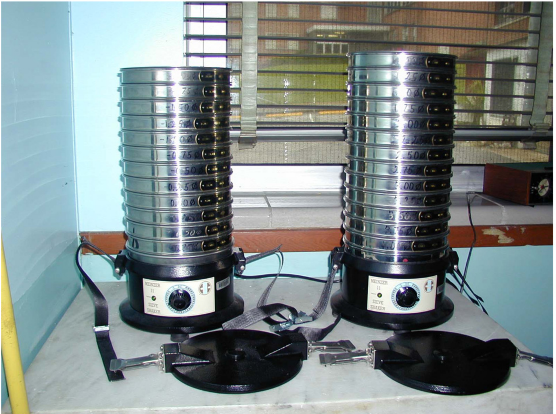
Figure 8. Sieve Nest Used in Processing Sediment Samples
