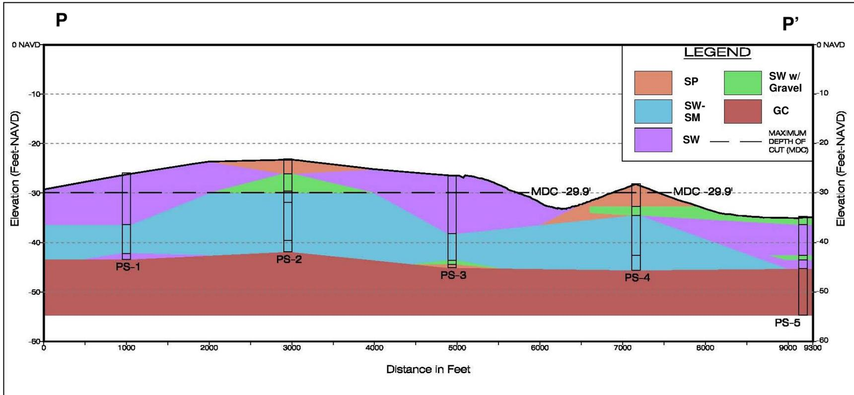
Figure 5.4: Pierce Shoal – Interpreted Fence Diagram
