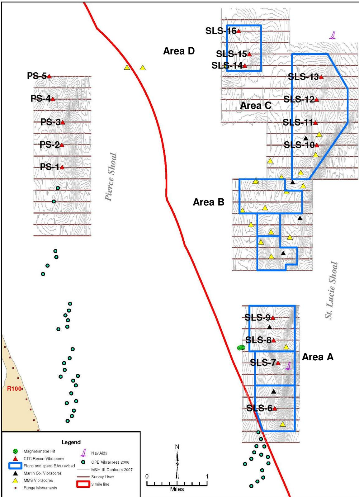
**Figure 5.1: Vibracore Locations and Potential Borrow Area Boundaries**
