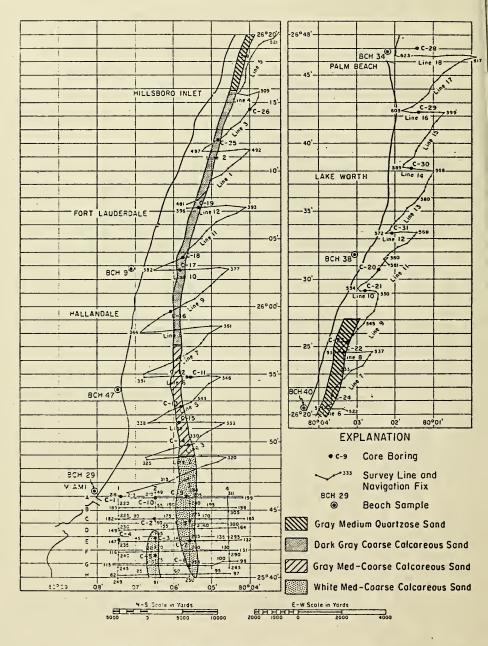
Figure 19. Areas most suitable for sand borrow.
