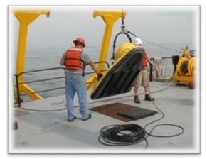
Figure 8: Image of the sub-bottom profiler 512i towfish.
