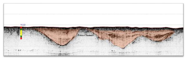
Figure 15: BOEM chirp sub-bottom Line 047, with plotted color coded vibracore FL-BOEM-2015-VC22 with highlighted digitized paleochannels.
