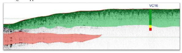
Figure 14: Chirp sub-bottom Line 042 offshore St. Johns County. The brown line at the top of the sub-bottom record represents the seafloor. Layers color coded as green are likely beach compatible, yellow indicates potentially incompatible material, and red indicates likely incompatible material. The color-code criteria are further explained in the Reconnaissance Geologic Sample Data Interpretation section of this report.
