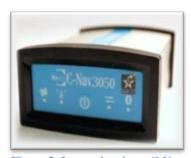
Figure 5: Image showing a C-Nav 3050 DGNSS receiver
