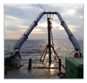
Figure 12: Alpine vibracore rig.
