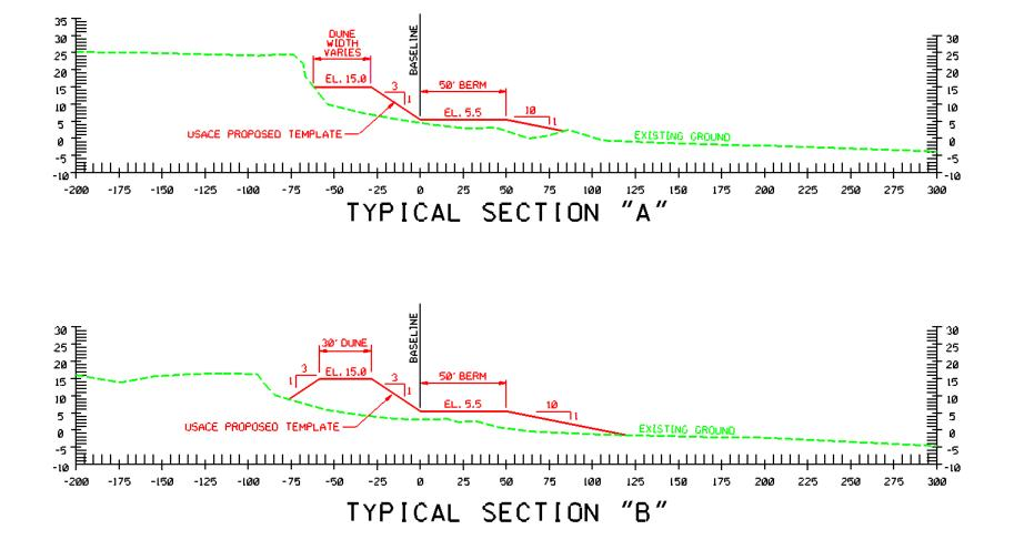
FIGURE B-6. TYPICAL PROJECT SECTIONS TO BE CONSTRUCTED
