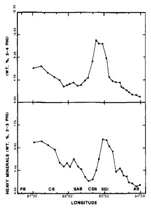
Fig.3. Four-point moving averages  $(2-3 \phi)$ , transect averages;  $3-4 \phi$ , individual samples) of weight percent heavy minerals versus longitude. PB — Pensacola Bay; CB — Choctawhatchee Bay; SAB — St. Andrews Bay; CSB — Cape San Blas; SGI — St. George Island; and AB — Apalachee Bay.
