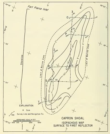
Figure 32. Isopachous Map of Sediment Thickness between the Water-Sediment Interface and the First Underlying Acoustic Reflecting Surface in the Capron Shoal Area.
