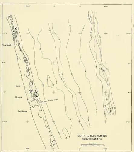
Figure 8. Contour Map of the Surface of the Blue Acoustic Reflector.
