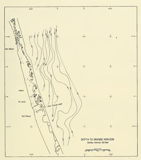
Figure 11. Contour Map of the Surface of the Orange Reflecting Horizon.
