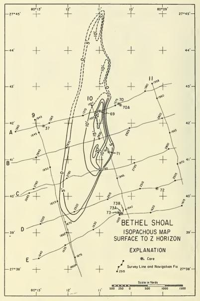
Figure 28. Isopachous Map of Sediment Thickness between the Water-Sediment Interface and the "Z" Horizon Underlying Bethel Shoal.
