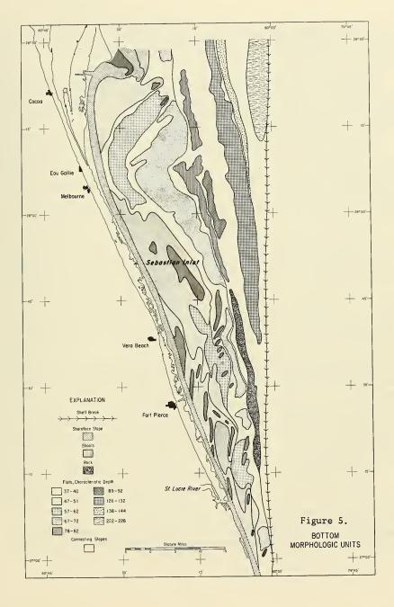
c. <u>Inner-Shelf Plain</u> - The inner-shelf plain is characterized by its extremely gentle seaward inclination, narrow depth range (nearly all the area is between -40 to -70 feet MLW) and its general alignment parallel to the northwesterly trend of the shoreline.
