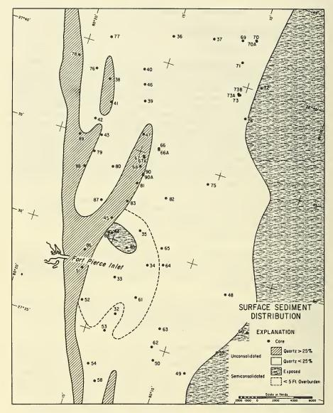
Figure 21. Generalized Map of the Surface Sediment Distribution in the Fort Pierce Grid Area.
